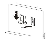
2 If applicable, set the XR Battery Enclosure **DC Disconnect** circuit breaker to OFF.
